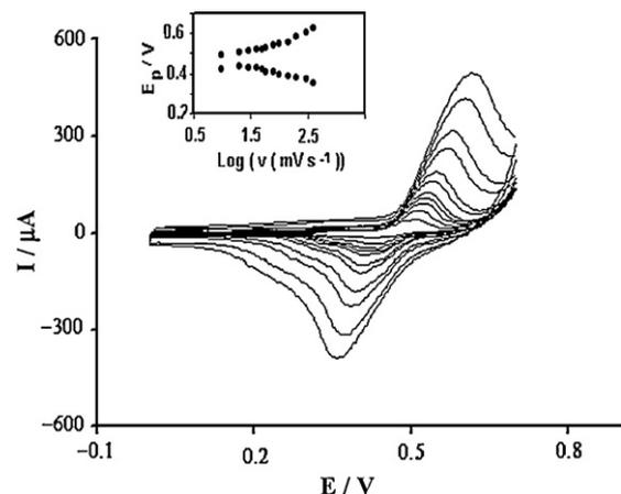
**Fig. 3.** Main panel: cyclic voltammograms of Ni/POA/CPE in  $0.1 \text{ mol L}^{-1}$  NaOH solution. Potential sweep rates from inner to outer are: 10, 20, 30, 40, 50, 80, 100, 150, 200, 300 and  $400 \text{ mV s}^{-1}$ . Inset: plot of  $E_p$  versus  $\log v$  for cyclic voltammograms depicted in the main panel.
