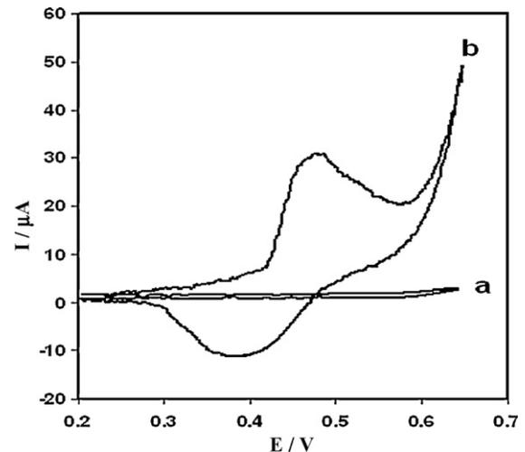
**Fig. 2.** Electrochemical responses of electrodes: (a) POA/CPE and (b) Ni/POA/CPE, in  $0.1 \text{ mol L}^{-1}$  NaOH solution, scan rate  $10 \text{ mV s}^{-1}$ .
