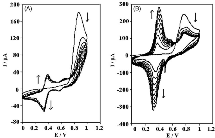
**Fig. 1.** Electropolymerization of POA in the solution of  $5 \text{ mmol L}^{-1}$  OA monomer/ $0.5 \text{ mol L}^{-1}$   $\text{H}_2\text{SO}_4$  at the surface of carbon paste electrode (A) in the absence and (B) in presence of  $5 \text{ mmol L}^{-1}$  SDS at scan rate of  $100 \text{ mV s}^{-1}$ . The arrows indicate the trends of current during CVs.
