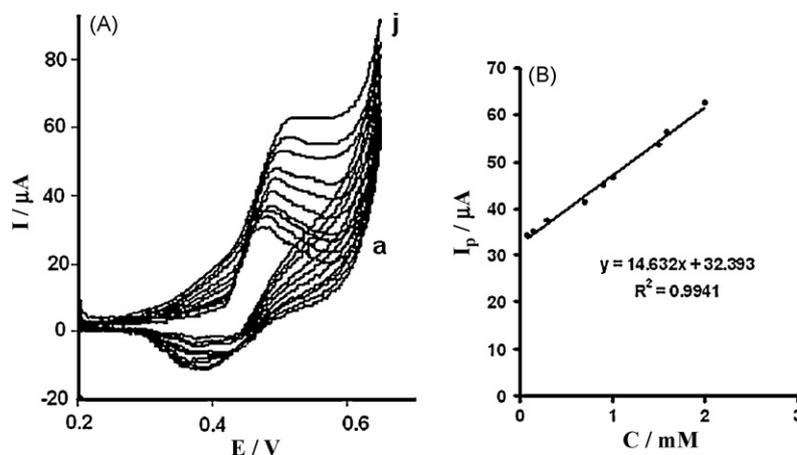
**Fig. 8.** (A) Current–potential curves for oxidation of cefixime at the Ni/POA/CPE in 0.1 mol L<sup>-1</sup> NaOH solution with different concentrations of cefixime: (a) 0 mmol L<sup>-1</sup>, (b) 0.08 mmol L<sup>-1</sup>, (c) 0.15 mmol L<sup>-1</sup>, (d) 0.3 mmol L<sup>-1</sup>, (e) 0.7 mmol L<sup>-1</sup>, (f) 0.9 mmol L<sup>-1</sup>, (g) 1 mmol L<sup>-1</sup>, (h) 1.5 mmol L<sup>-1</sup>, (i) 1.6 mmol L<sup>-1</sup> and (j) 2 mmol L<sup>-1</sup>. (B) Plot of  $I_p$  versus  $c$ .
