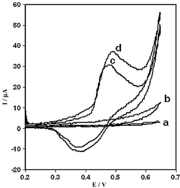
**Fig. 4.** Electrochemical responses of POA/CPE prepared in the presence of SDS to: (a) 0 mmol L<sup>-1</sup>, (b) 0.3 mmol L<sup>-1</sup> cefixime and Ni/POA/CPE to: (c) 0 mmol L<sup>-1</sup> and (d) 0.3 mmol L<sup>-1</sup> cefixime in 0.1 mol L<sup>-1</sup> NaOH solution, scan rate 10 mV s<sup>-1</sup>.
