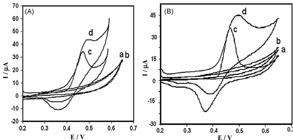
**Fig. 5.** (A) Electrochemical responses of POA/CPE to: (a) 0 mmol L<sup>-1</sup>, (b) 0.3 mmol L<sup>-1</sup> ceftriaxone and Ni/POA/CPE to: (c) 0 mmol L<sup>-1</sup> and (d) 0.3 mmol L<sup>-1</sup> ceftriaxone in 0.1 mol L<sup>-1</sup> NaOH solution, scan rate 10 mV s<sup>-1</sup>. (B) Such as (A) for cefprozime.
