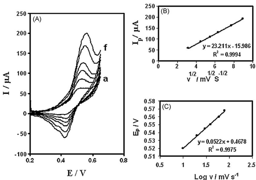
**Fig. 6.** (A) cyclic voltammograms of the Ni/POA/CPE in 0.1 mol L<sup>-1</sup> NaOH solution containing 1.5 mmol L<sup>-1</sup> cefixime at the scan rates: (a) 10 mV s<sup>-1</sup>, (b) 20 mV s<sup>-1</sup>, (c) 30 mV s<sup>-1</sup>, (d) 40 mV s<sup>-1</sup>, (e) 60 mV s<sup>-1</sup> and (f) 80 mV s<sup>-1</sup>, respectively. (B) Variations of  $I_p$  versus  $v^{1/2}$ . (C) Dependence of the peak potential,  $E_p$  on  $\log v$  for the oxidation of cefixime at Ni/POA/CPE.
